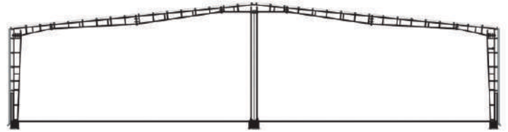
MULTI SPAN FRAME WITHOUT CRANE
