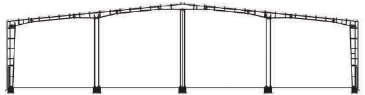
MULTI SPAN FRAME WITHOUT CRANE
